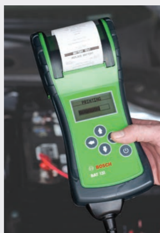
BAT 131 with integrated printer. The graphical printout includes detailed test results.
