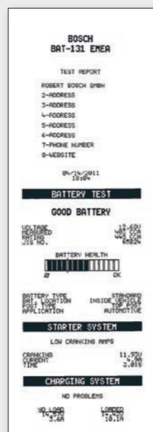
BAT 131 with integrated printer. The graphical printout includes detailed test results.
