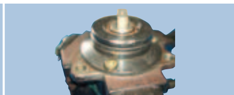
Heavy mechanical damage on drive flange or shaft
