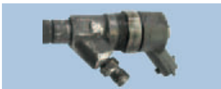
Heavy mechanical damage
