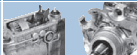
Incomplete or dismantled pump
