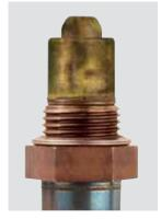
**Lambda sensor condition:**Green, grainy soiling
