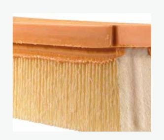
Poor processing, low-quality sealing material
