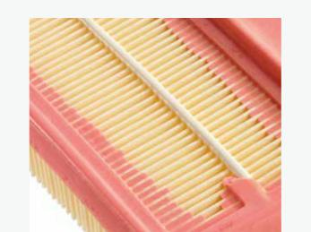
Excessive use of sealing material
