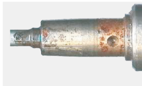
Corrosion at the injector
