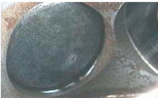
Corrosion at the high-pressure pump housing
